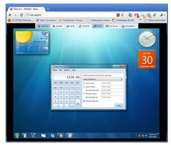
ThinVNC works on any HTML5-compliant web browser and does not require any additional plugin, add-on or installation of any kind on the client side. ThinVNC exploits HTML5 canvas to display a remote PC desktop, taking full advantage of WebSockets, AJAX, JSON and HTML5 technologies.
