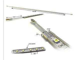
Installation of this Light Bar is extremely simple. Every bar includes two mounting clips, and each clip is attached to the surface with one screw. LED light bars can be powered with a plug-in 12V Adapter or a hard-wired 12V Indoor/Outdoor driver with the use of our waterproof connectors.
