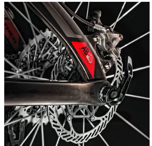
US PATENT #7,837,213 — TREK'S ACTIVE BRAKING PIVOT (ABP)
