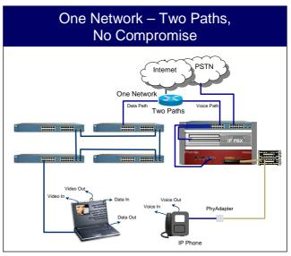
wire with reach of 1,200 ft. The new, more customer-centric paradigm is having one network, two paths. The existing data path for data and IP enabled voice path leveraging the existing voice infrastructure
