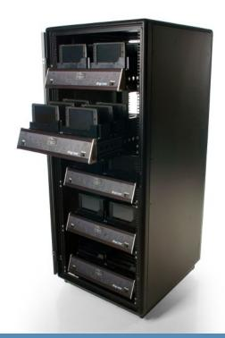
Making content loading easier, we offer a content update station that uses POE, so no battery, to load 100 digEplayer L7s simultaneously. The station requires only a small space.
