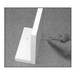
**STEP 10** Use the 1/4"-20 x 1-1/4" bolts, 1/4" washers, and 1/4"-20 3 point knobs to mount the stop blocks to the jig.
