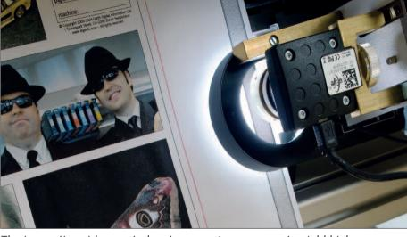
The innovative video control system uses two cameras to yield high-precision, front-to-back registration – without operator intervention.
