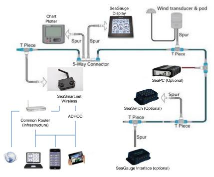
Chetco Digital SeaSmart.Net™ technology makes wireless gauge viewing, data access and data storage as easy as using a smart phone and browser. SeaSmartWiFi is bundled with sample Web Pages for instant setup. Custom development tools are also included.
