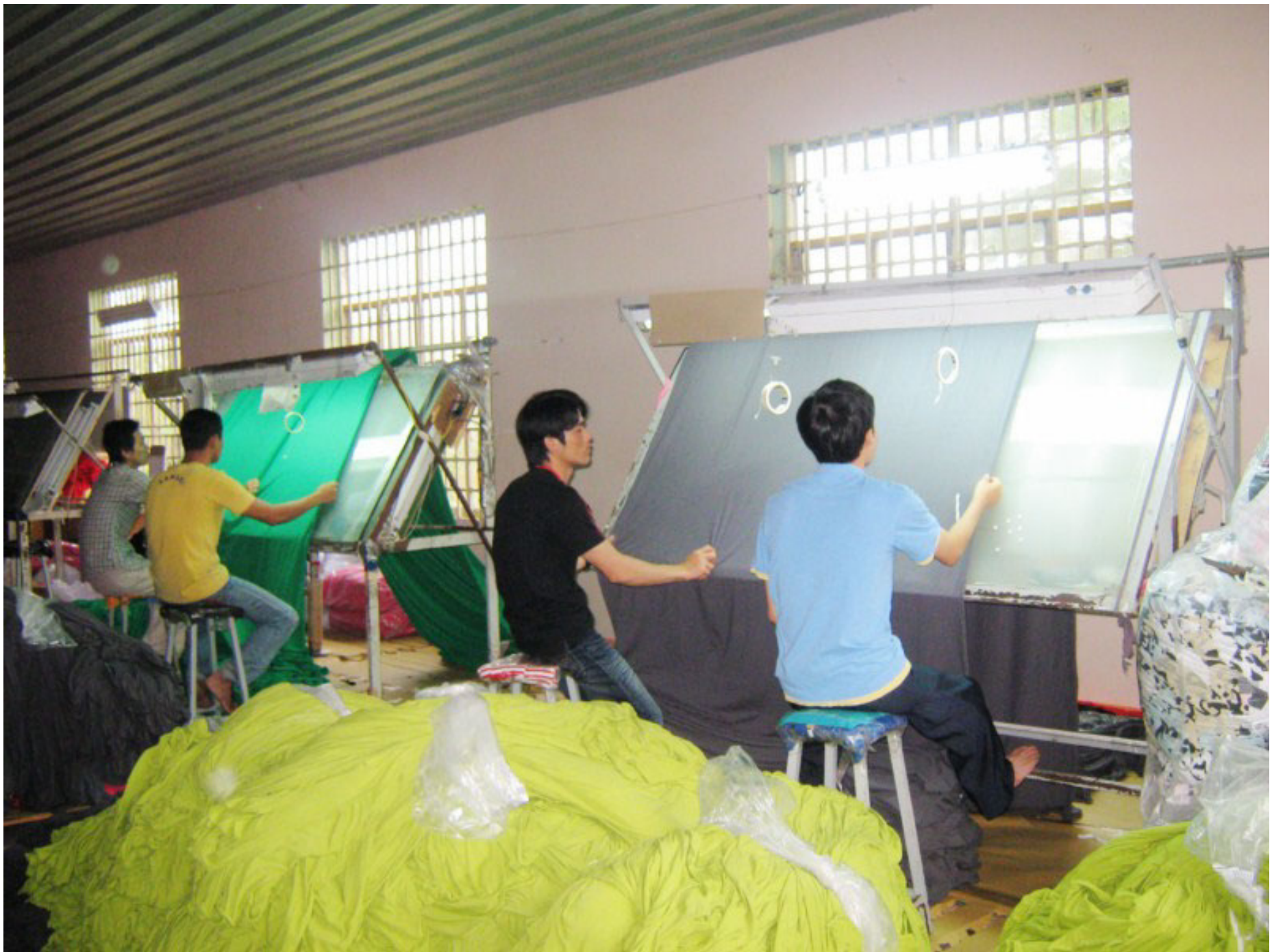
14 Fabric checking area
