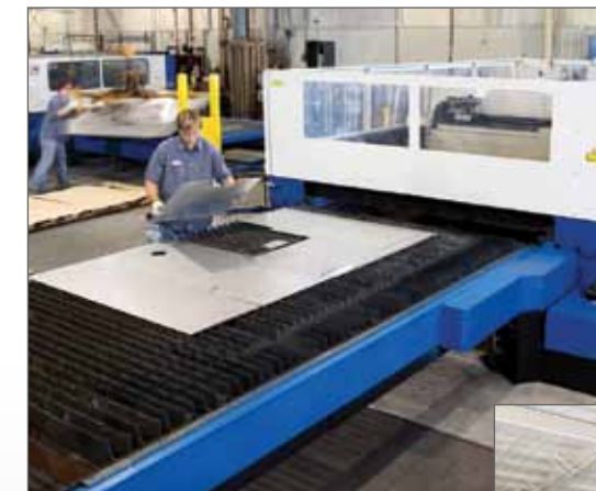
Integrated, in-house manufacturing systems include MRP-linked laser tables to ensure highly accurate sheet and plate cutting for tight fit and quality finish.
