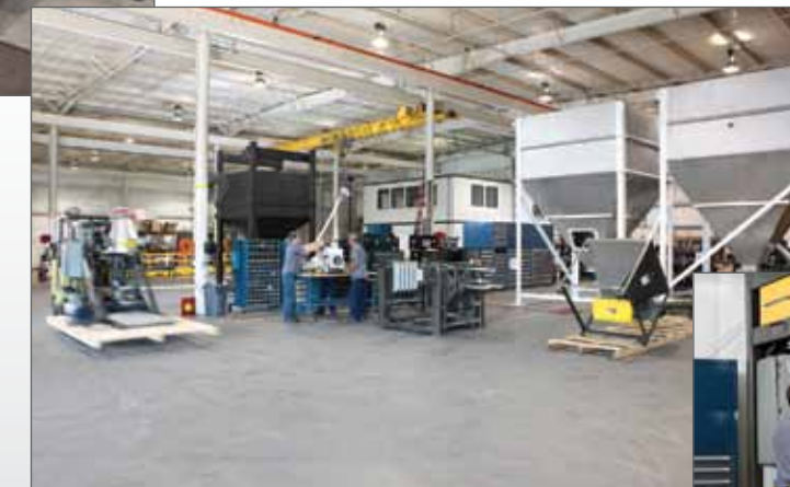
Multiple, large-scale factory acceptance testing areas enable complete, pre-installation set-up, operation, and customer evaluation of equipment and automation prior to shipment, installation, and start-up.
