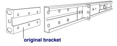
3. Input rear long bracket to rear of the rail then adjust rear bracket to fit your cabinet. Tight-up 2~3 screws upon the length you need. One is forbidden.
