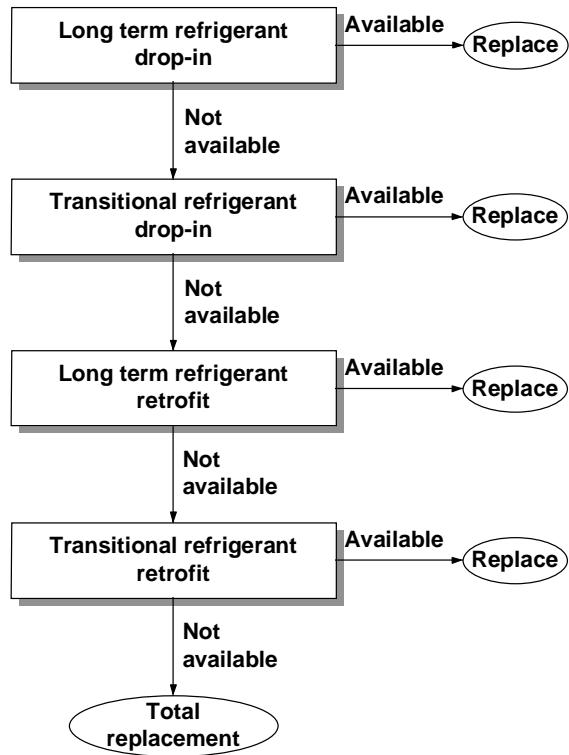
Applying the logic of Figure 4 to the table of R12 alternatives in Figure 5a gives the following results (the following logic could equally be applied to R22 and its alternatives in Table 5b):
