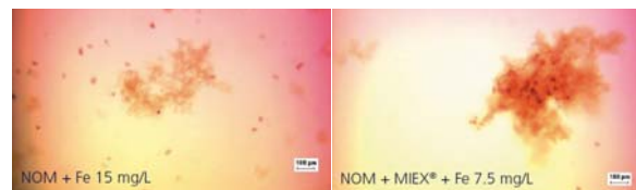
Figure 1: Example of flocs formed from Albert Raw Water with: 15mg/L Fe (left), MIEX® Pretreatment and 7.5mg/L Fe (right)
