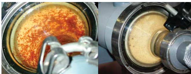
Figure 2: UF membrane backwash after pretreatment with in-line coagulation (left) versus MIEX® Pretreatment (right)
