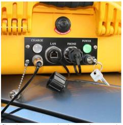
Since the case never needs to be opened to operate, it can be used in any extreme location. The external power cable is connected, and the LAN watertight cap is removed to show an Ethernet jack.
