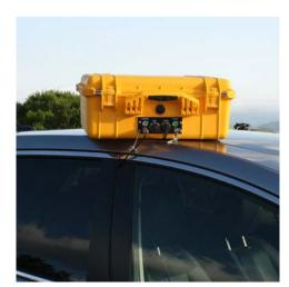
The Football requires line of sight to one of three stationary BGAN satellites so placing it on top of a car avoids blocking a signal. If this case were secured to a roof rack, the car may be moving and stay connected.
