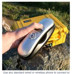
the case phone (RJ-11) port. We recommend a phone that does not require external power to function. There is room inside of the case to store items such as a phone as the one shown above.
