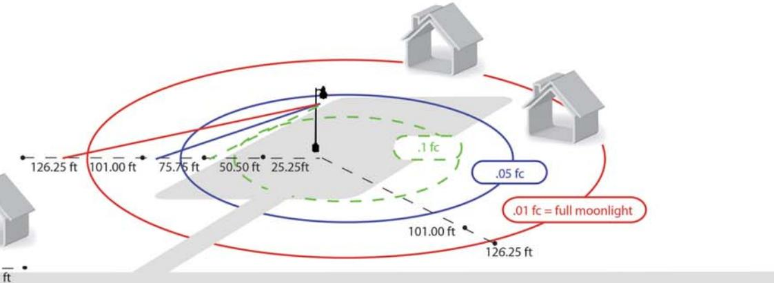
The 50W Clearlight Beacon delivers .01 fc (full moonlight) at over 4 mounting heights per side making it the perfect replacement lamp in legacy MV or HPS fixtures used as streetlights, parking lot lights, barn lights or general area lighting.
