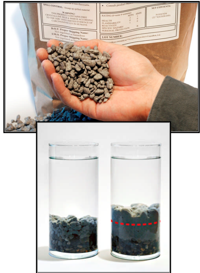
Figure 1. Configuration of stone-clay composite particle.
