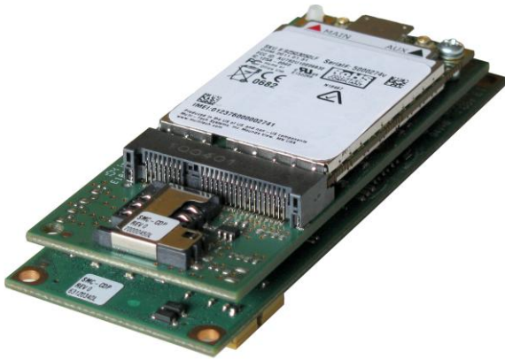
Fig. 1: MultiConnect™ OCG-E is a complete wireless Linux applications engine in a small 3.7" x 1.4" outline
