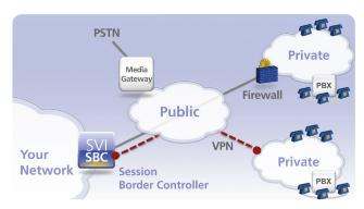
This cost effective SBC provides unified or distributed signalling deployment while securing the network boundary from comprehensive Denial Of Services (DOS), registration throttling and authorization overload with comprehensive firewall protection including subscriber authentication and policy enforcement. Focused session management capabilities are controlled using the industry leading Graphic User Interface (GUI) which simplifies the process of securing and managing your network border.
