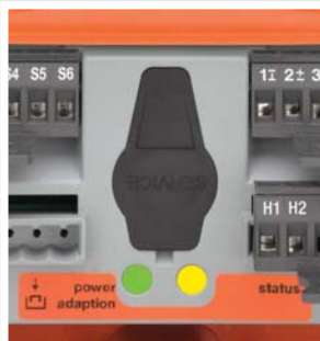
MFT interface socket with LED indicators.
