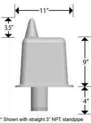
\* Shown with straight 3" NPT standpipe to fit the 0°, 5°, 10°, 15°, 20°, and 30° mounting flanges
