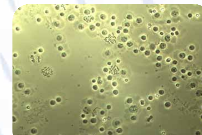
Image of cell spots generated by the BioDot AD1500 (Olympus BX40 Phase Microscope, Phase 2, 10X objective). This slide surface was increased to 30°C.
