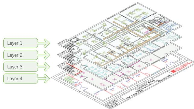
Unlike other CAD to PDF solutions who flatten the file when converting to PDF, the Adlib CAD Module maintains optimal file integrity by preserving the layers encoded in the original CAD file.
