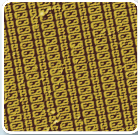
Microstructure. Scan size 30x30 \mu\text{m} . Semicontact mode
