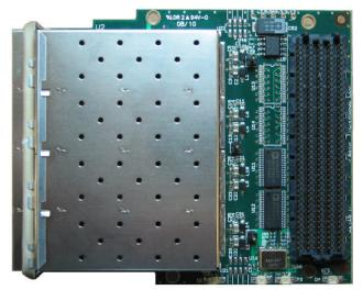
The FM-S14 is electrically compliant with the FMC standard. Due to the size of the quad SFP cage, the FM-S14 is classified as a mechanical superset of the FMC mechanical standards. Special attention should be paid to ensure that the FM-S14 is mechanically compatible if used with non-supported host carrier cards.
