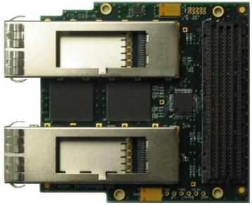
cards. The FM-S28 is electrically compliant with the FMC standard. Due to the size of the QSFP cages, the FM-S28 is classified as a mechanical superset of the FMC mechanical standards. Special attention should be paid to ensure that the FM-S28 is mechanically compatible if used with non-supported host carrier cards.
