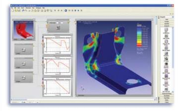
Fast and direct simulations of shaker tests in the frequency domain
