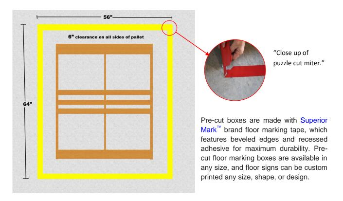
Note: This floor marking kit is designed to mark a border around a standard pallet. Standard pallets measure 40" x 48", and this kit leaves a 6" clearance on all sides of the pallet. Available in 2" and 4" widths, can be custom made to create any size box.
