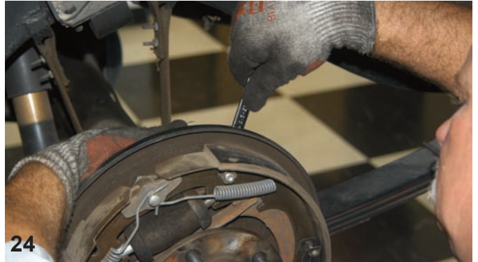
Using a long box-end wrench the bolts that connect the backing plate to the axle were removed.
