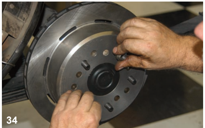
The special 11-inch rotor that works with the internal parking brake mechanism was installed. Three lug nuts were installed to check the caliper to rotor centering.
