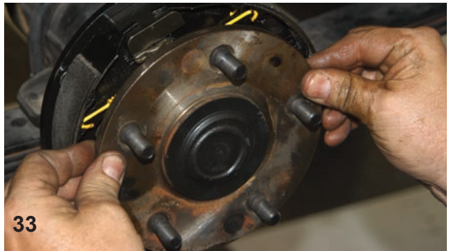
The axle was spun in the housing to make sure there was no interference and then the axle flange face was cleaned with a wire brush to remove any debris.
