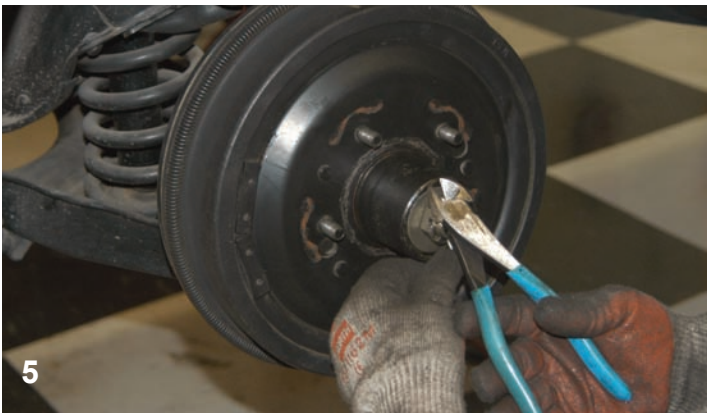
The cotter key was removed from the nut to spindle connection. Here the cotter key is being removed with cutting pliers.
