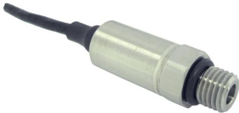
Measurement Specialties, Inc. (NASDAQ: MEAS) has just released its new [EB100](#) pressure transducer for production. It is CE compliant and offers a pressure range of 300 to 5000psi (350bar) and operates from -40°C to +125°C with a ±1% TEB. This high accuracy, [miniature device](#) was specifically designed for space-constricted designs in motorsports, military/aerospace, off-road, industrial, test stand and hydraulic applications.
