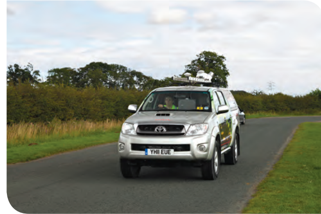
Dynascan road survey in progress
