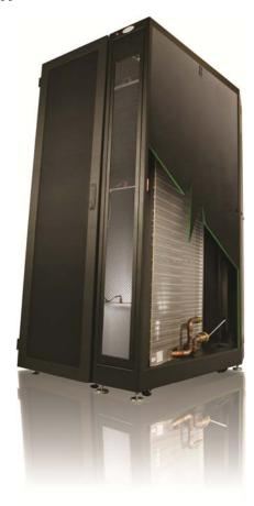
coil provides increased cooling capacity for higher density loads. In addition, because of the larger coil, warmer water could be used to economically cool 20+kW heat loads, reducing the load on the chiller and providing further energy cost savings while maintaining the same cooling capacity of a standard Coolcentric RDHx. In many cases this could also allow the use of Free Water Cooling (evaporator water), a source of cooling with significantly reduced energy cost.
