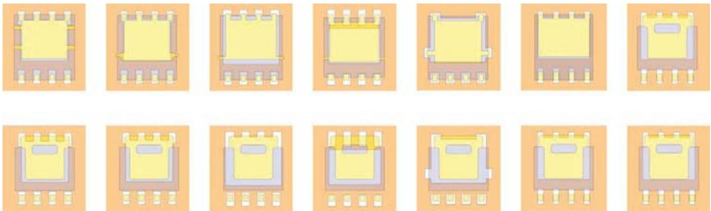
Through careful design of the PCB footprint, it is possible to design a universal footprint, such as the one shown below, that meets the requirements of various Power-SO8 manufacturers. The example universal footprint shows the solder resist & solder stencil details, which allow a PCB designer to create a footprint that is compatible with other Power-SO8 vendors.
