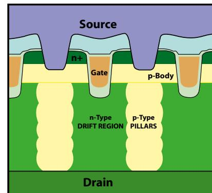
NextPower technology uses p-Type pillars to improve the breakdown voltage in the OFF state, and a heavily doped n-Type drift region to achieve exceptionally low ON resistance.
