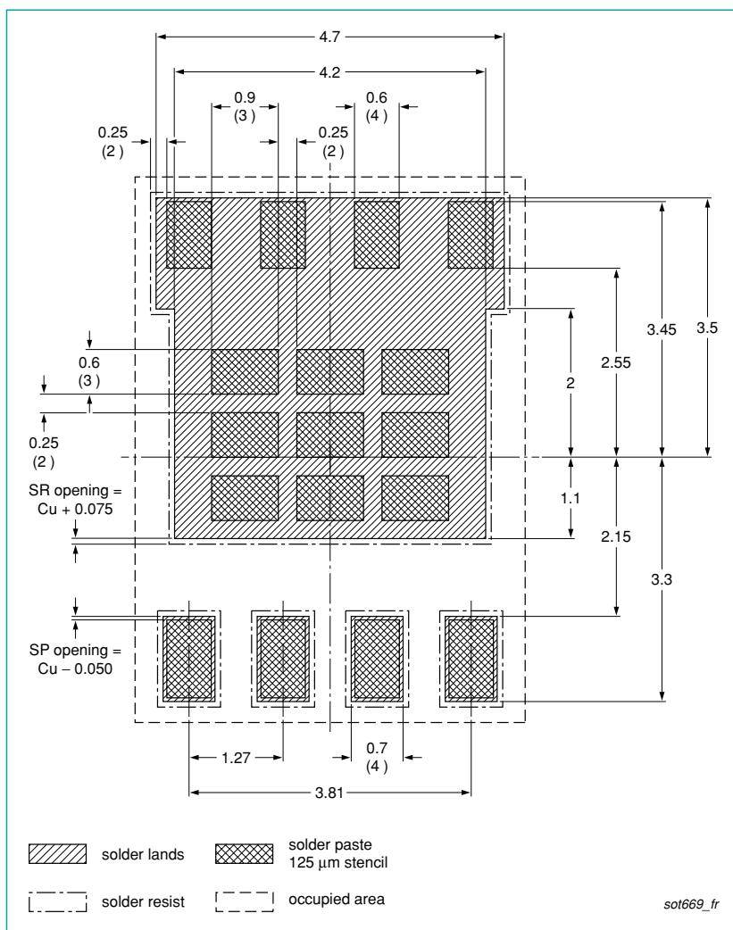
Recommended universal Power-SO8 & LFPAK footprint allows the following device types to be mounted to a single PCB design:
