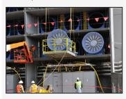
IBHS researchers conducted a wind test demonstration in fall 2010 that pitted a conventionally constructed house (below) against a house built to IBHS' FORTIFIED Midwest construction standards (right) in winds nearing 100 mph, only the FORTIFIED house survived.
