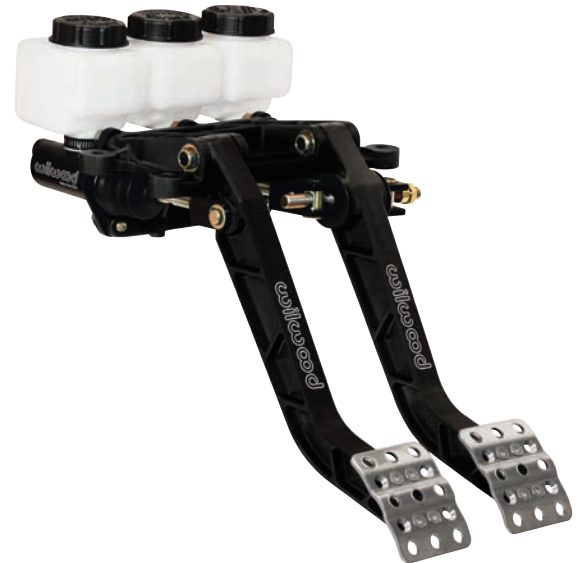
Forward Mount Pedal Assembly Shown with Optional Master Cylinders
