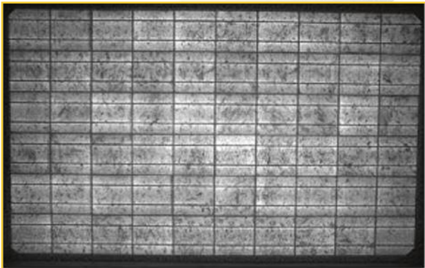
Magnified 'C' grade cell after 10 years of production.
