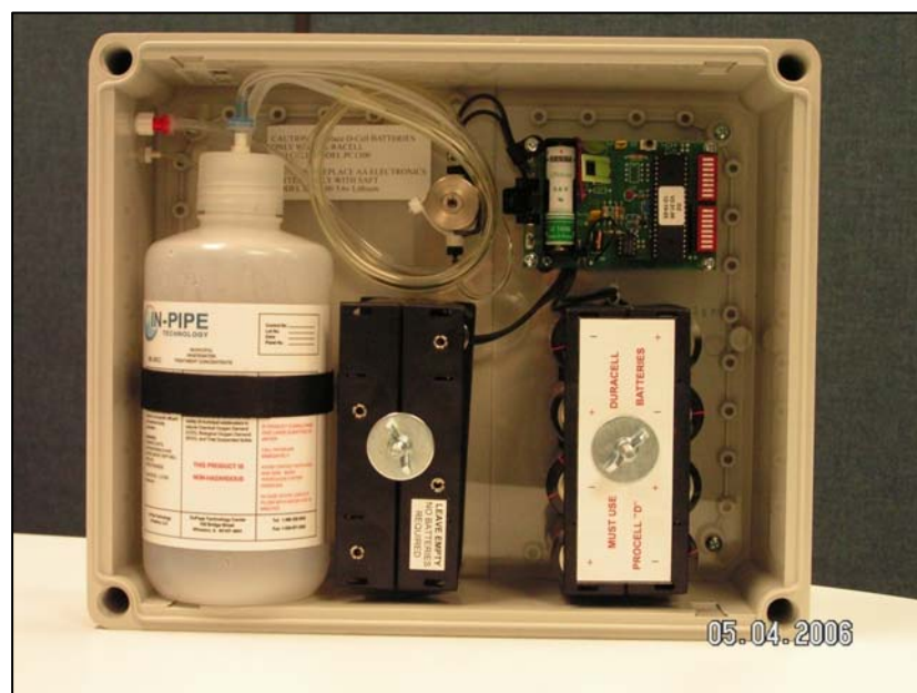
Figure 2 – Bioaugmentaion Dosing Panel
