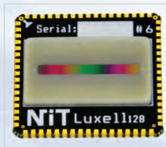
LUXELL 128 FPA WITH LVF INCORPORATED Main applications are measurements with spectral discrimination
