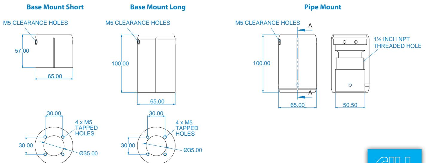
All options are supplied with appropriate fixing screws and washers.
