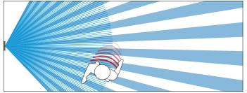
This is the most common type of motion sensor. PIR sensors monitor the patterns of background heat energy in a given space. That is, if you sit still for a long time, the sensor will think of your static heat signature as a normal condition and return to "Off" mode. When movement of a heat source is detected the sensor turns "On". When the sensor does not detect the heat source movement it returns to "Off" mode. PIR sensing technology is great for avoiding false triggers.
