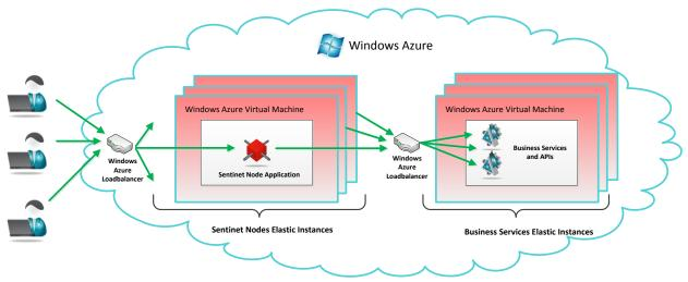
Sentinet Nodes can be deployed as native Windows Azure Cloud Services Web Roles or Virtual Machines, <u>http://www.windowsazure.com/en-us/develop/net/fundamentals/intro-to-windows-azure/#models</u>.
