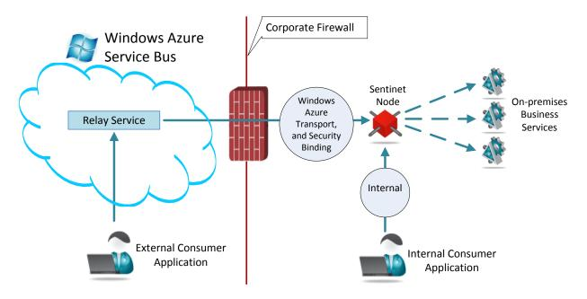
Sentinet Nodes can also be deployed in the hybrid deployment scenarious, where some Nodes are deployed on-premises while others are in the cloud. Both consumer and service applications can be fully decoupled (encapsulated) from Windows Azure Service Bus specific APIs and security configurations.
