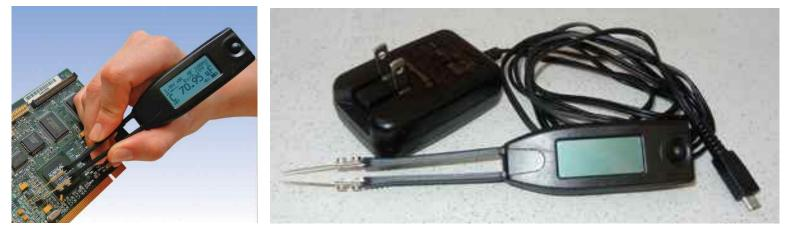
Smart Tweezers is a new patented design concept integrating a digital multimeter with a built-in gold-plated SMD probes and a display. This light weight device can be easily held by one hand. and is idealy suitable for component evaluation on a PCB or a production line and sorting of SMD components. Smart Tweezers dramatically reduces time necessary to troubleshoot or debug a PCB simplifying process of locating a faulty component.
