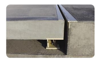
The Harvester® truck scale's factory-poured precast concrete decks are 7.25 inches thick for optimum strength, and the entire scale is only 14.75 inches high from the top of the pier to the top of the scale deck for a low profile.
