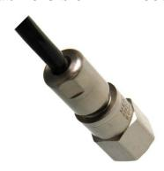
Measurement Specialties, Inc. (NASDAQ: MEAS) is now in full production of its Model 8042-01 Submersible IEPE Accelerometer certified for >100 meter depth. This sensor is available in ±10g, ±80g and ±500g dynamic ranges with an operating temperature range of -20 °C through +80 °C, non-linearity of ±1% and shock protection to 5000 g's.
