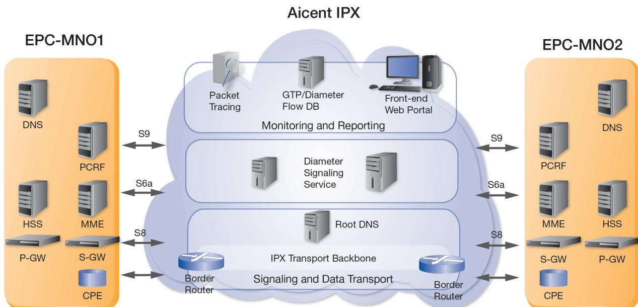
*Aicent IPX for LTE Roaming - IP connectivity and transport is provided between two LTE networks via Aicent IPX Transport*
