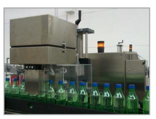
pressure value. Any container with internal pressure that falls below user set limits is rejected. The system is ideal for plastic containers and eliminates the need for unsanitary and expensive squeeze belts. The system is also ideal for glass containers with aluminum or steel closures such as beer and sparkling wines.
