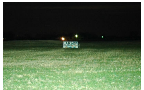
This image shows a close up picture of the 'Larson' sign, notice that the beam output still reaches farther than the sign positioned 750 feet away from the unit.
