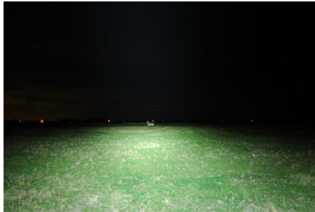
This photo shows the LEDPB10W-120X2E. In flood configuration, the light passes the 'Larson Electronics' Sign more than 750 feet away, yet still provides a large width for work area illumination.
