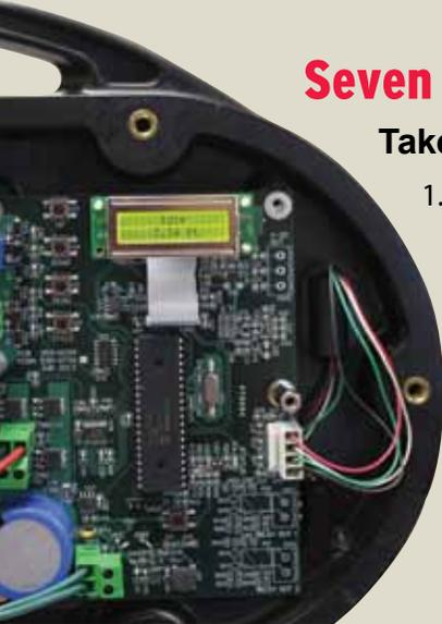
The SmartBob AO level sensor requires standard 115 VAC or 230 VAC power. There are two current source options for supplying power. The recommended option is to use an isolated 4-20 mA current loop which uses the PLC to provide power. Alternatively, a non-isolated 4-20 mA current loop can utilize the SmartBob sensor to provide power for the loop.
