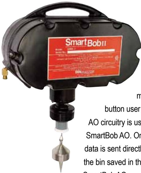
The SmartBob AO level sensor features an integrated 4-20 mA analog output for use by facilities that prefer an analog output to a PLC for monitoring bin level measurement data. A simple push-button user interface built into the SmartBob AO circuitry is used to configure the settings for each SmartBob AO. Once setup is complete, measurement data is sent directly to a PLC, with all settings for the bin saved in the non volatile memory of the SmartBob AO.
