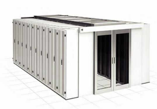
In this example, CPI Aisle Containment Doors are combined with a Cabinet Supported Ceiling Panel Kit and the F-Series TeraFrame® Cabinet System to enclose the cold aisle between adjacent cabinet rows. The overhead ceiling traps cold air in the aisle so that it will be used to cool equipment, instead of the entire room.
