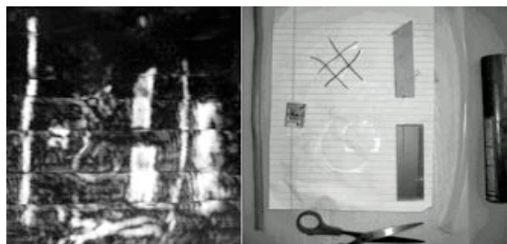
Figure 10. Wire, metal, wood and plastic (14-3 wire, 30GA #, pine board, HDPE pipe, copper pipe, small PCB, 30GA wire loop, PCB, scissors)
