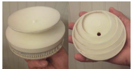
Figure 5. Antenna assembly (left) and FZP element (right)
