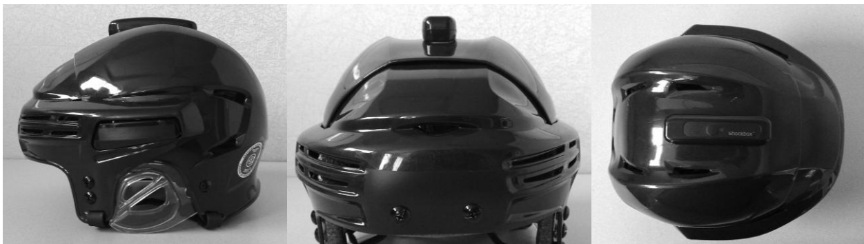
Fig. 1. Position of impact sensors attached to exterior crown of standard hockey helmets.
